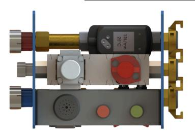
Automated surveillance of air pressure, flow rate, and outlet water temperature. Any irregularity promptly activates an audible and visual alarm (insufficient pressure, low flow rate, or overheating).
